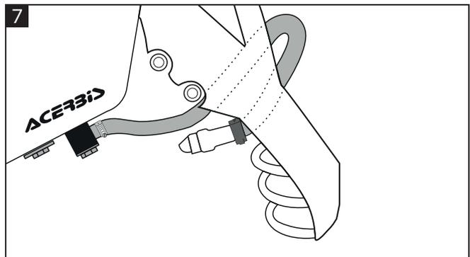
**Attach the HUSQVARNA fuel line to the Acerbis tank (A) as indicated in the diagram. Make sure the fuel line isn't folded over, obstructing the fuel flow.**
