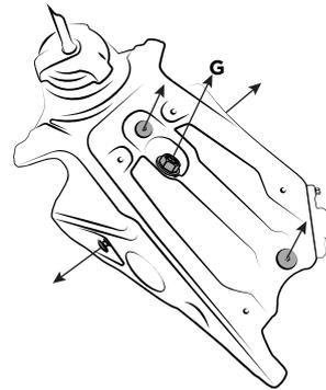
**Empty any remaining fuel from original fuel tank. Remove the seat, side panels and radiator scoops. Remove the screws that fixing seat and radiator scoops. Remove the screw tank (G).**
