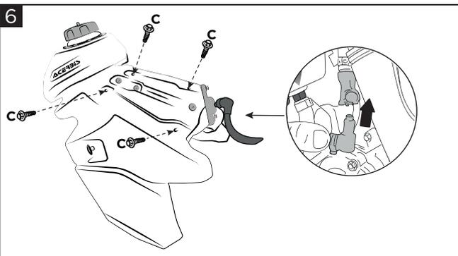
**Reconnect the fuel pump power cable and the fuel connector. Remount the side panels through the screws (C), the radiator scoops and the seat.**
