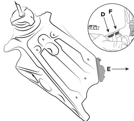
**Remove the pump (E) and the fasteners (D/F) from the original tank.**
