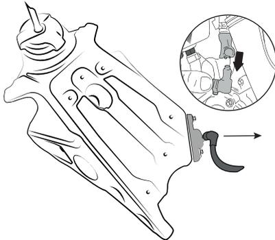
**Disconnect the fuel pump cover cable and the fuel connector as indicated in the diagram. Remove the original tank.**
